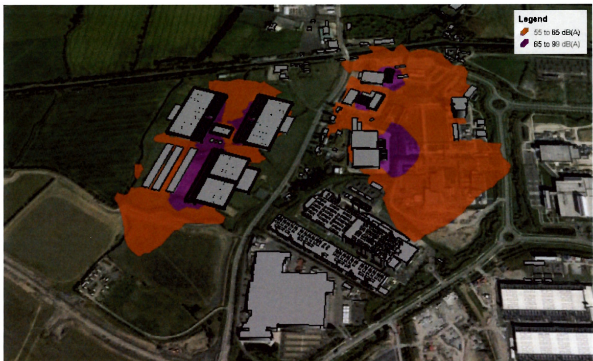
Figure 9.7 Scenario B – Noise contour – emergency operation (with all generators)
